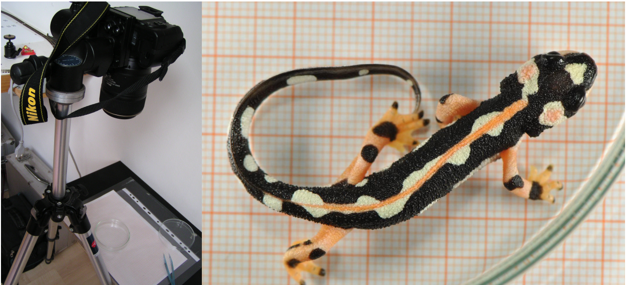
Abb. 2: Camera set-up for photodocumentation with a Nikon D3000, AF-S Micro Nikkor 105 mm, Nikon SB-900, 2 Nikon SBR-200, tripod with tripod head Manfrotto 410 (left) and an example of an animal photographed from the dorsal perspective (animal 38).
